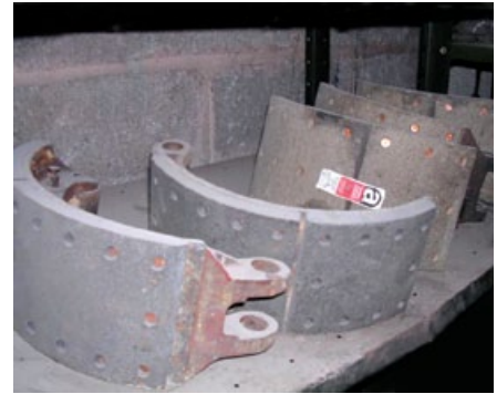
Figure 41 Asbestos brake linings for quarry vehicles
